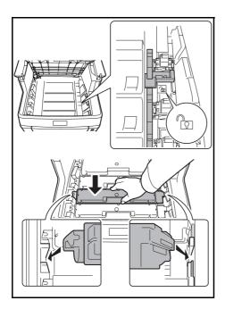
4 Make sure the release lever is in the release position and set the new toner container in the machine.
